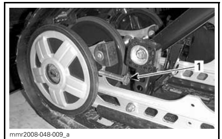
1. RH adjustment screw
