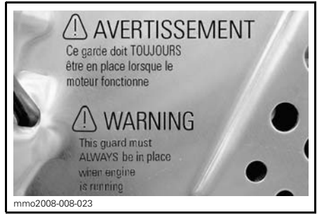
LABEL 17 - ON BRAKE DISC GUARD (BARE METAL TUNNEL)
