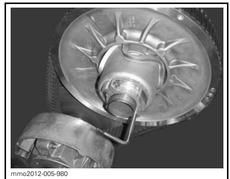
PULLEY EXPANDER INSTALLED ON ADJUSTER HUB
