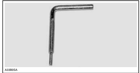
DRIVE BELT INSTALLER/REMOVER TOOL
