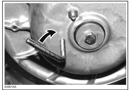
DRIVE BELT INSTALLER/REMOVER TOOL
