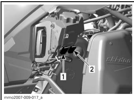
TYPICAL 1. 30 A charging system fuse 2. 5 A start/RER fuse
