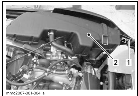
1. Air filter 2. Air silencer
