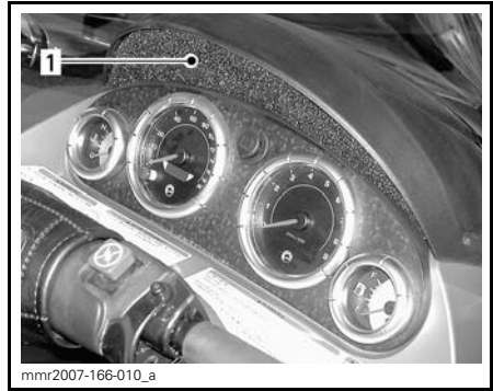
TYPICAL 1. Air filter installed in air inlet duct
