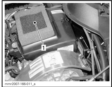
1. Air filter installed on top of air silencer
