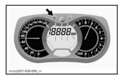
While display flashes, press the SET (S) button to select top speed (TOP\_SPD) mode.
