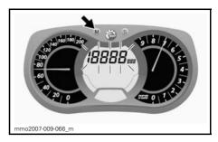
While display is flashing, press the SET (S) button to select speedometer mode.
