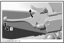
TYPICAL — RELEASE MECHANISM Step 1: Squeeze brake lever
