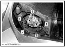
Step 1: Push both sides in Step 2: Pull to release
