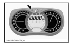
While display flashes, press and hold the SET (S) button within 5 seconds to reset.
