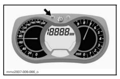
To reset maximum temperature recorded, press the MODE (M) to select mode.
