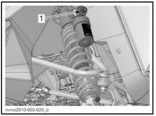
High speed compression damping adjuster (hexagonal)
