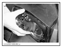
Disconnect burnt bulb connector. Remove the rubber boot.
