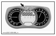
While display flashes, press the SET (S) button to select total fuel consumption (TC) mode.
