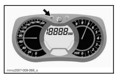
To reset, set the trip meter to TRIP B. Refer to TRIP METER "A" OR "B" for more details
