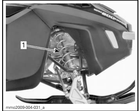
TYPICAL - FRONT SUSPENSION 1. Front springs for handling
