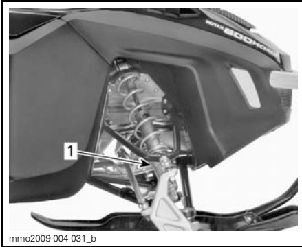
TYPICAL - CAM TYPE PRELOAD 1. Adjustment cam
