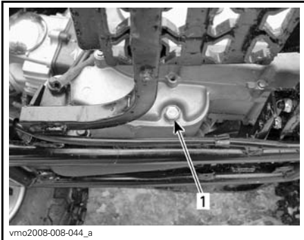
LH SIDE OF ENGINE 1. Drain plug
