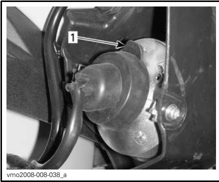
REMOVE RUBBER PROTECTOR 1. Rubber protector
