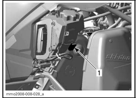
TYPICAL - RH SIDE OF ENGINE COMPARTMENT 1. 5 A start/RER fuse
