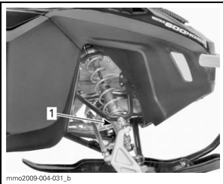
TYPICAL - CAM TYPE PRELOAD 1. Adjustment cam
