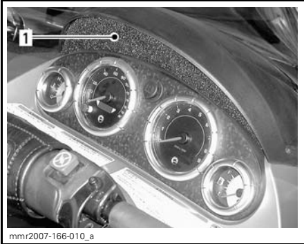
1. Air filter installed in air inlet duct
