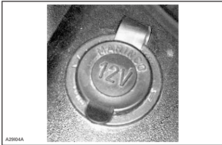
TYPICAL — ELECTRIC POWER OUTLET
