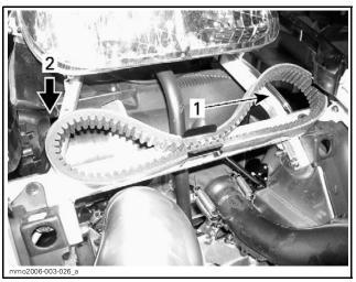
SPARE DRIVE BELT INSTALLED IN HOLDER
