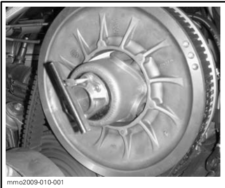
EXPANDER INSTALLED ON SCREW TYPE DRIVEN PULLEY
