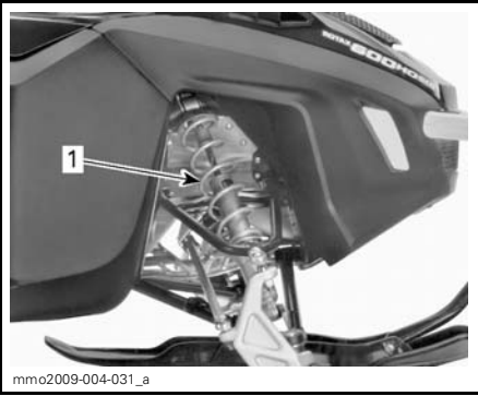
TYPICAL - FRONT SUSPENSION 1. Front springs for handling
