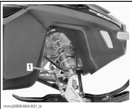
TYPICAL - CAM TYPE PRELOAD 1. Adjustment cam
