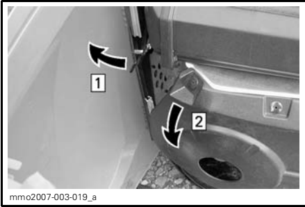
Step 1: Push on tab Step 2: Pull on belt guard to remove
