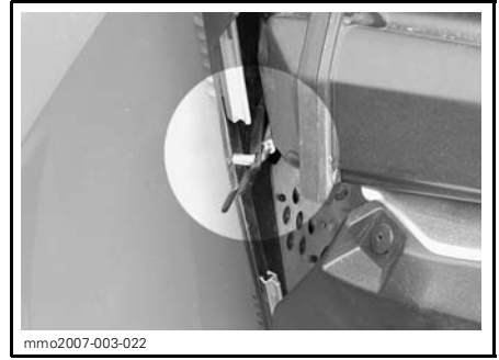
FRONT RETAINING PIN PROPERLY SECURED
