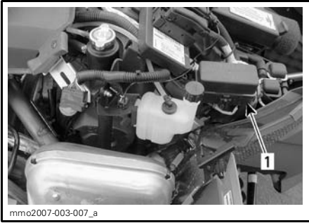
RH SIDE OF VEHICLE 1. Fuse box
