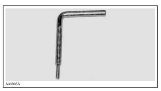
PROPER TOOL TO BE USED ON MX Z X 440
