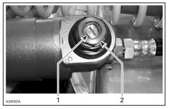
1. Low speed compression adjuster (flat screwdriver)
