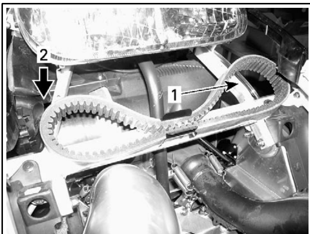
FAN COOLED — SPARE DRIVE BELT INSTALLED IN HOLDER
