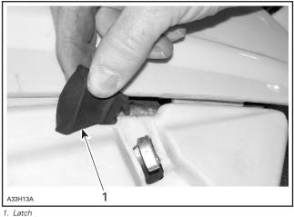
To remove a side panel remove by pulling up both locking devices from hinge.
