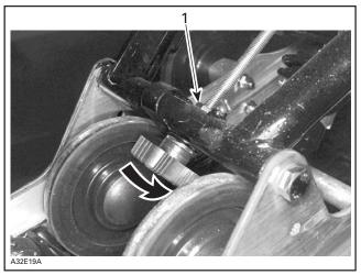
1. Loosen lock nut, turn knob accordingly then retighten lock nut
