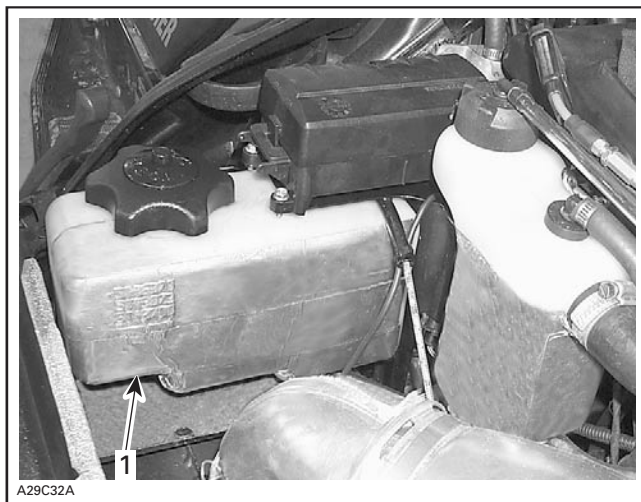
1. Injection oil reservoir
