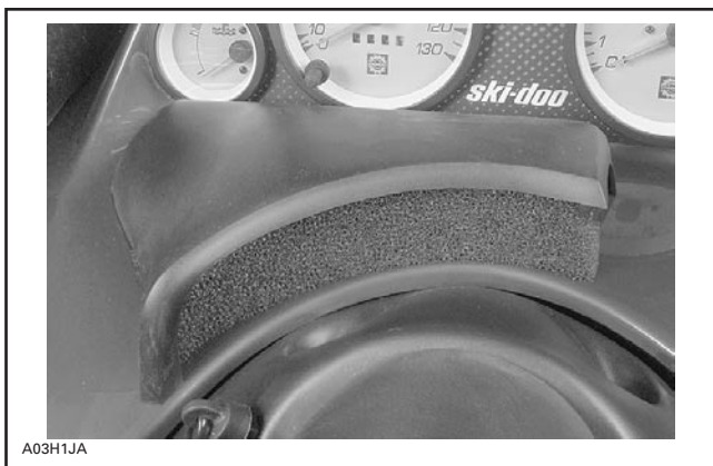
TYPICAL — FILTER INSTALLED
