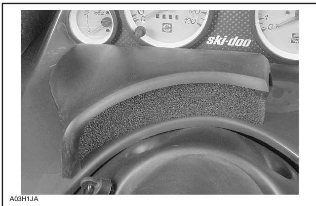
TYPICAL — FILTER INSTALLED
