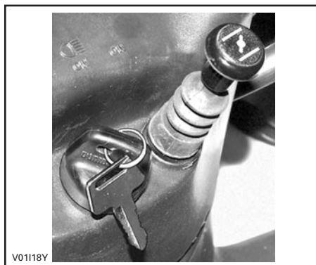
CHOKE LEVER IN THE FULL CHOKE POSITION
