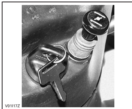
CHOKE KNOB LEVER IN THE OFF POSITION
