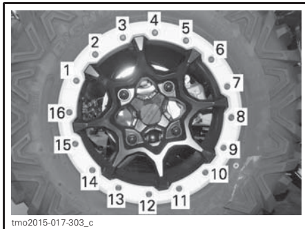
TYPICAL - FINAL TIGHTENING SEQUENCE
