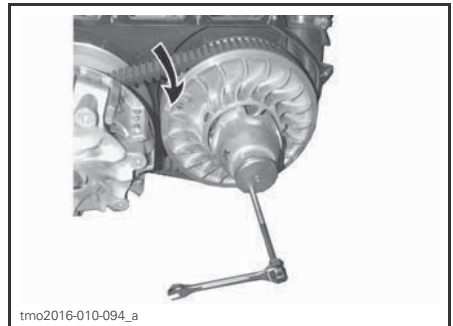
tmo2016-010-094_a TYPICAL Drive Belt Installation
