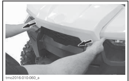
PULLING ON FRONT SERVICE COVER EDGE.
