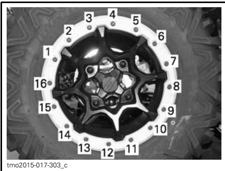
TYPICAL - FINAL TIGHTENING SEQUENCE
