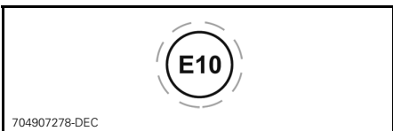
LOCATED NEAR GAS CAP
