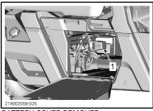
BATTERY COVER REMOVED 1. Rear fuse box
