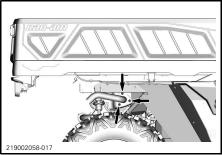
TAIL PIPE RETAINING SCREWS
