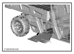
Remove battery cover by unscrewing the two 1/4 turn fasteners.
