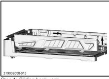
Step 1: Sliding backward Step 2: Lifting up
