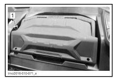
To open tool box, unlock panel and lift lid.
