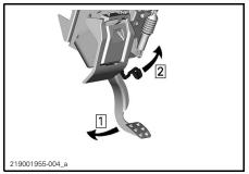
Step 1: Apply and hold brake pedal Step 2: Lift lever
