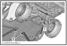
Lifting location under trailer hitch
