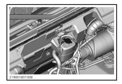
3. Unscrew coolant drain plug and drain the coolant into a suitable container.
