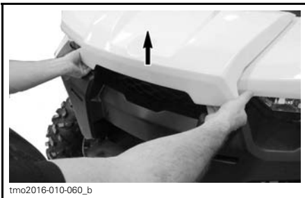
tmo2016-010-060_b LIFTING FRONT SERVICE COVER EDGE.
