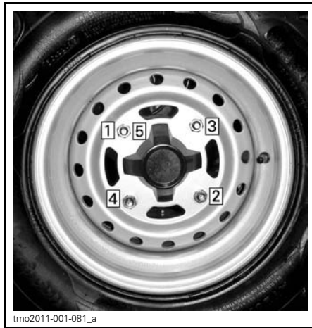
TIGHTENING SEQUENCE
