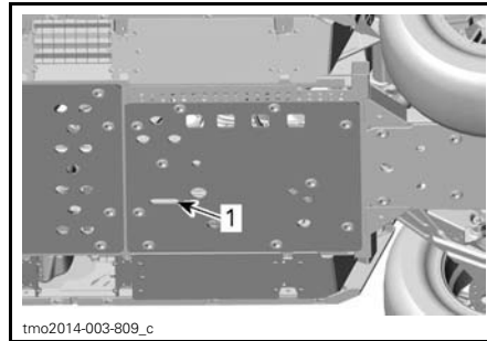
1. Cooling system drain plug access
