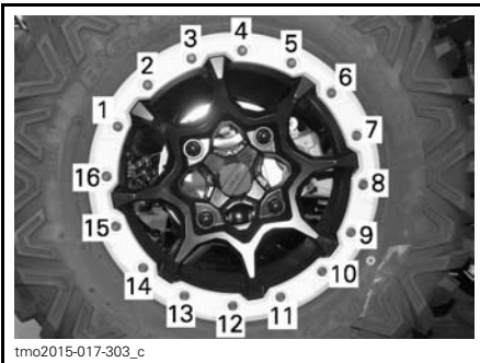
TYPICAL - FINAL TIGHTENING SEQUENCE
