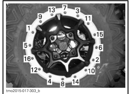
TYPICAL - TIGHTENING SEQUENCE
