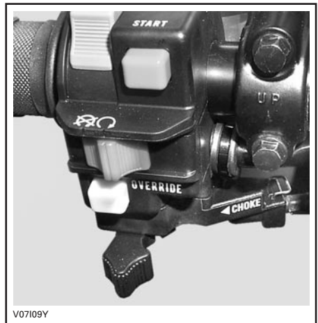
CHOKE LEVER IN THE FULL CHOKE POSITION
