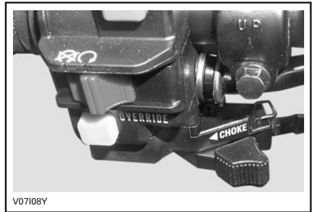
CHOKE LEVER IN THE OFF POSITION
