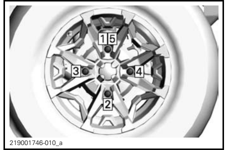
TIGHTENING SEQUENCE
