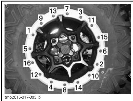
TYPICAL - TIGHTENING SEQUENCE
