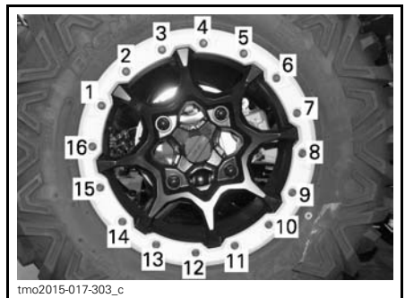
TYPICAL - FINAL TIGHTENING SEQUENCE
