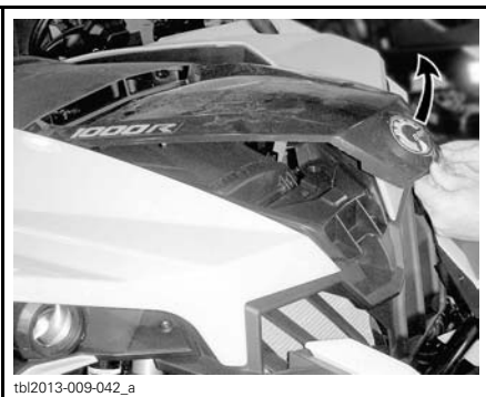
Step 1: Keep on lifting the front part of service cover Step 2: Gently release the cover post from its grommet then release the post on the other side
