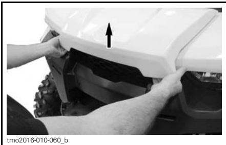
LIFTING FRONT SERVICE COVER EDGE.
