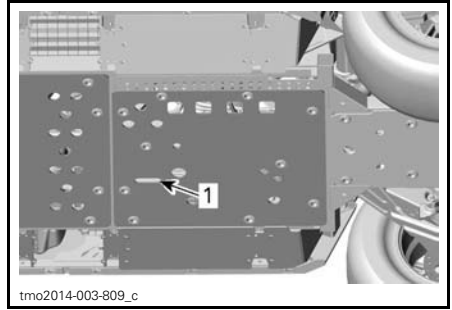
1. Cooling system drain plug access
