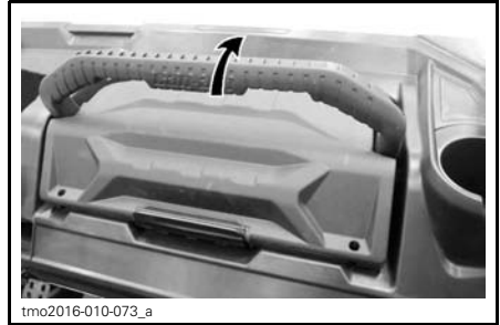
SECURING TOOL BOX IN PLACE
