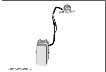
FUSIBLE LINK CONNECTED TO FUSE BOX
