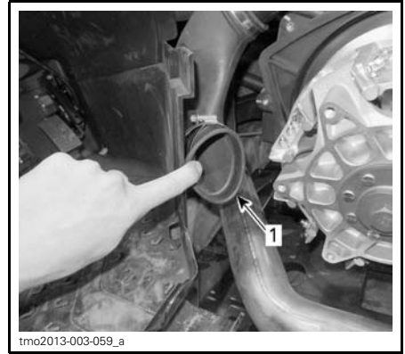
TYPICAL 1. Inside CVT outlet hose
