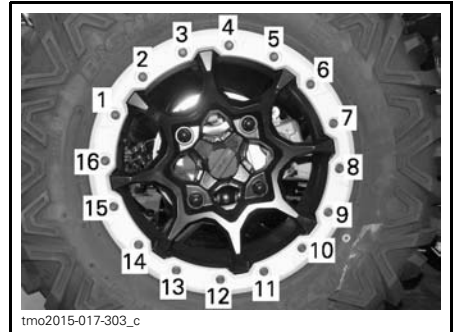
TYPICAL - FINAL TIGHTENING SEQUENCE
