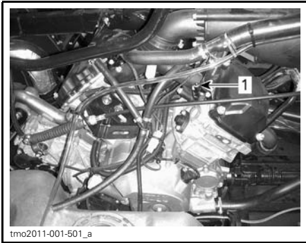
1. Front cylinder bleed screw
