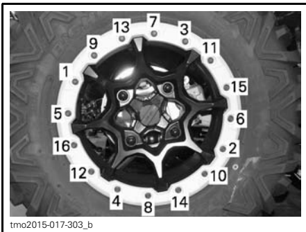
TYPICAL - TIGHTENING SEQUENCE
