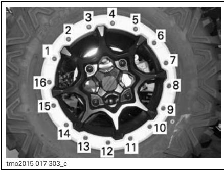
TYPICAL - FINAL TIGHTENING SEQUENCE
