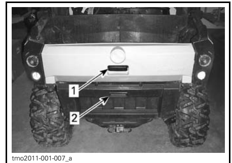
1. Cargo box upper section 2. Cargo box lower section
