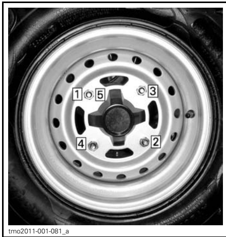
TIGHTENING SEQUENCE
