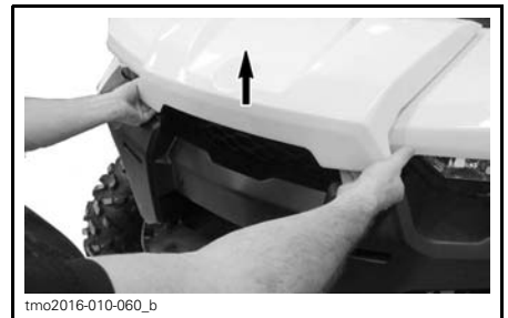
LIFTING FRONT SERVICE COVER EDGE.
