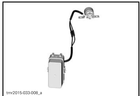
FUSIBLE LINK CONNECTED TO FUSE BOX
