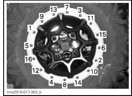
TYPICAL - TIGHTENING SEQUENCE
