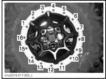
TYPICAL - FINAL TIGHTENING SEQUENCE
