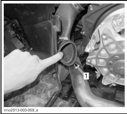
TYPICAL 1. Inside CVT outlet hose
