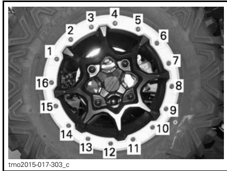
TYPICAL - FINAL TIGHTENING SEQUENCE
