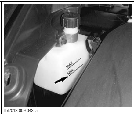
COOLANT EXPANSION TANK
