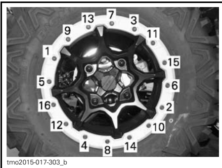
TYPICAL - TIGHTENING SEQUENCE
