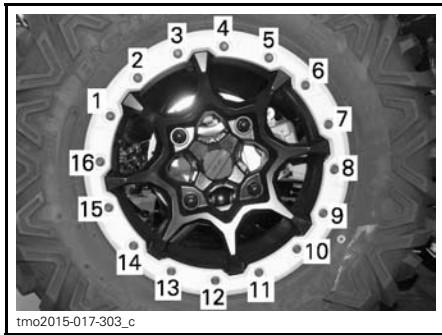
TYPICAL - FINAL TIGHTENING SEQUENCE
