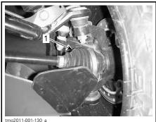
**FRONT OF VEHICLE** 1. Outer drive shaft boot
