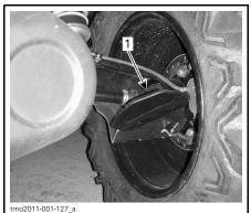
**REAR OF VEHICLE** 1. Outer drive shaft boot
