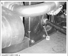
**REAR OF VEHICLE** 1. Inner drive shaft boot
