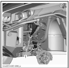
FRONT OF VEHICLE - COMPONENTS REMOVED FOR CLARITY 1. Front grill kit
