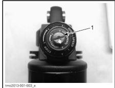
TYPICAL - XT-P MODEL 1. Low speed compression adjuster
