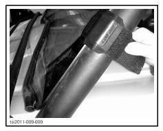
Install retaining screws in windshield and torque retaining screws to specification.
