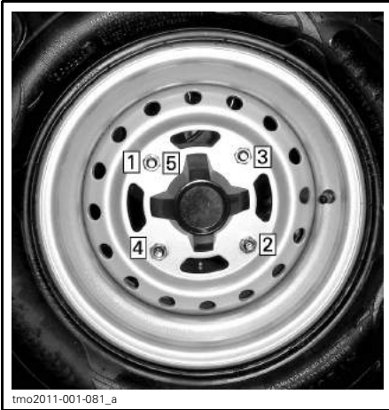
TIGHTENING SEQUENCE
